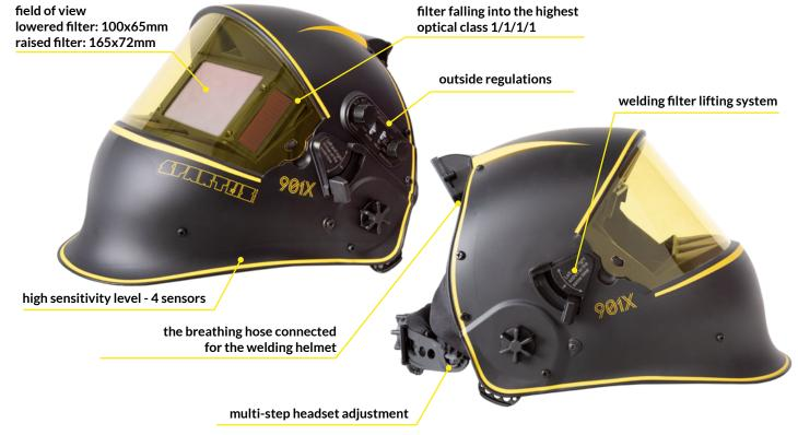
The multi-stage adjustment of the headgear allows not only a perfect fit, but also the right distance between the filter and the welder's eyes.
